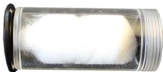
Fig. 8: Filter sleeve with cotton
