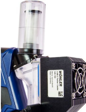
Fig. 3: Peltier cooler with cotton filter
