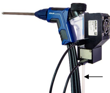
Fig. 5: Peltier cooler and Condensate pump mounted on probe handle, transparent condensate hose marked with an arrow
