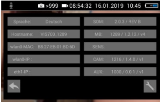
Fig. 7: Info menu with SOM (Firmware of the camera) and CAM (Version of the camera head)
