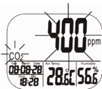
Fig. 21: Display during the CO 2 calibration
