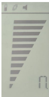
Fig. 15: Display shortly after switching on, automatic switch-off is deactivated
