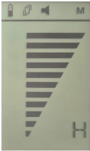
Fig. 18: Display with sensitivity set to high
