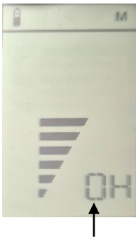
Fig. 17: Display during manual sensor zeroing
