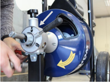
Fig. 10: Automatic feed unit marked by grey arrow
