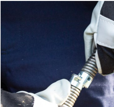
Fig. 4: Fixing the drill head with the snap-lock
