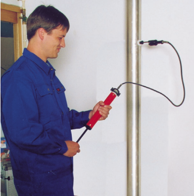
Fig. 3: Extracting the smoke gas
