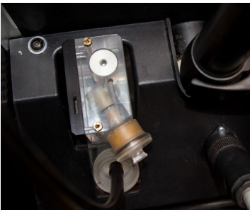
Fig. 2: Condensate trap module installed on gas path
