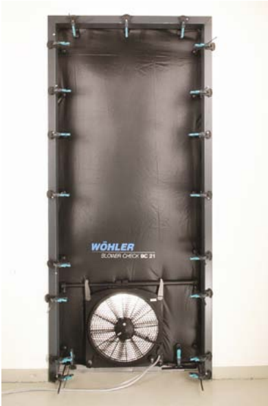
Fig. 15: Blower Unit and sealing film completely assembled.
