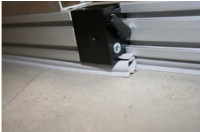
Fig. 14: The locking lever is sloped: The slide is blocked.
