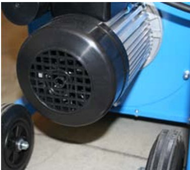
Fig 4: Motor with ventilation slots
